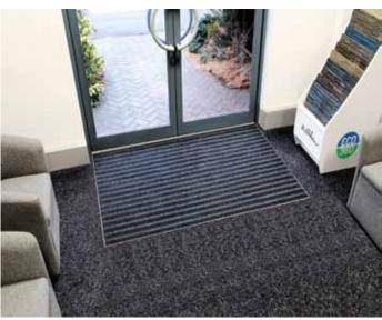
Rolls can be cut to the desired length to produce a tailor made mat or runner. This can be loose laid on the floor, or bonded to the subfloor using an acrylic tackifier adhesive.
